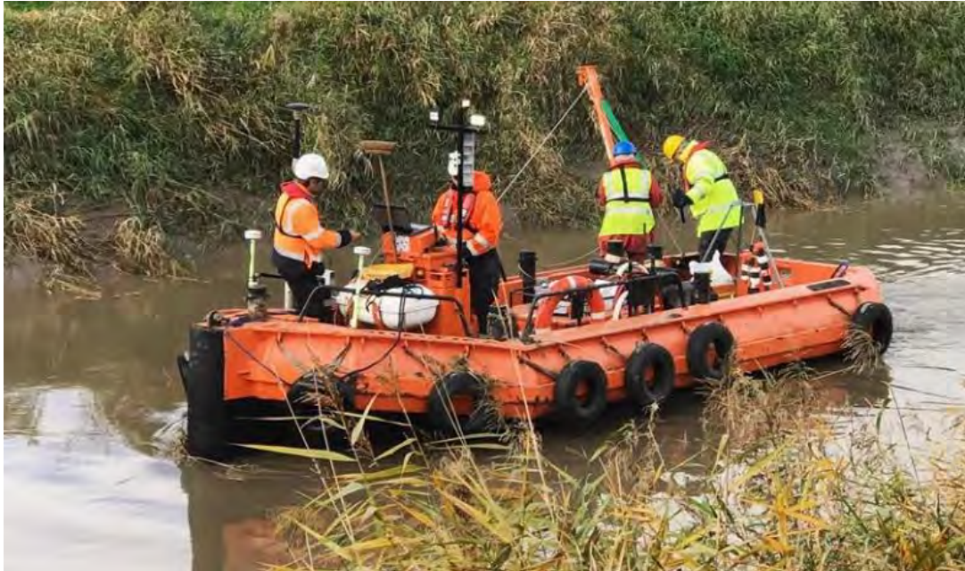
Figure 4. The CHALLIS 2 workboat showing the derrick used for the Owen tube.
