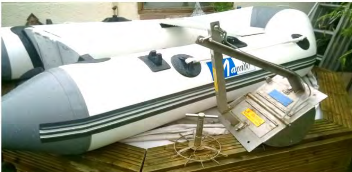
Figure 6. Inflatable dinghy, grab and shear vane used for the bed surveys.
