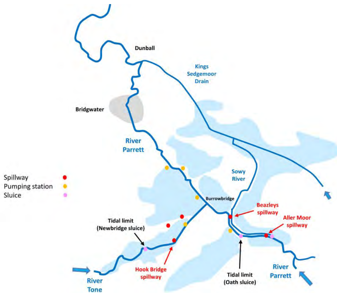
Figure 16. The Parrett and Tone: Drainage routes, spillways, pumping stations and water storage areas. The Severn Estuary is to the north (top).
