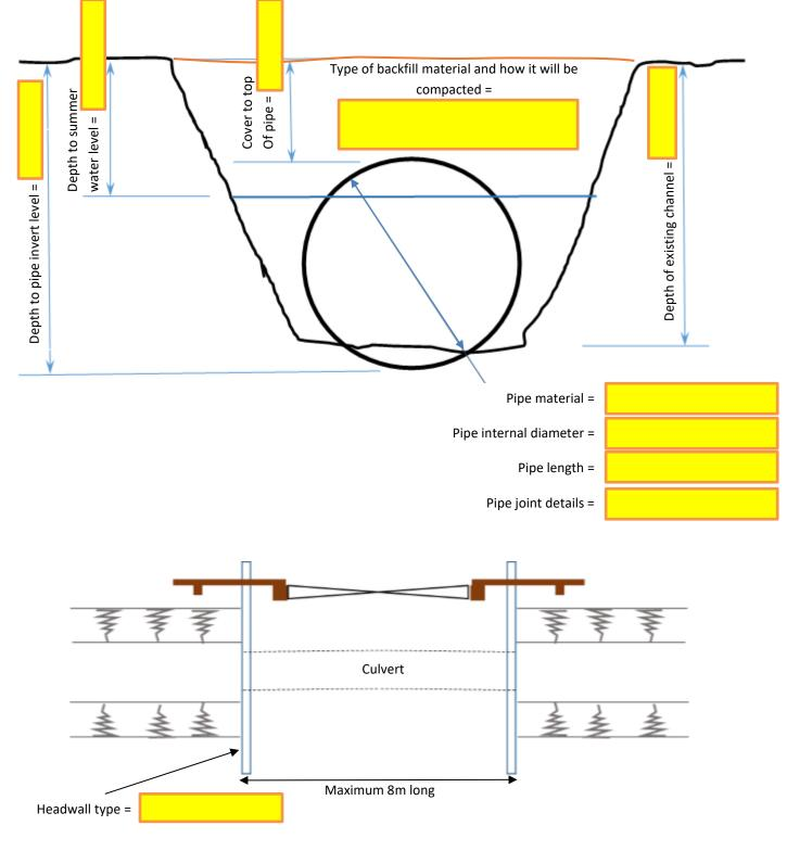
PLAN OF CHANNEL AND CULVERT
