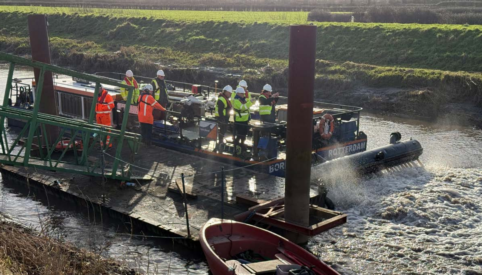
Above: Borr's water injection bar is raised for visitors from Lincolnshire. Below right: a screen in Borr's cabin shows the vessel's relation to the River Parrett's profile.
